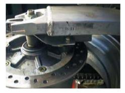
The **Speed Sensor** (7) is on the rear swing arm on the right side, and uses a bracket that is mounted on the rear axle. The magnets fit into the head of the bolts that mount the brake disc to the wheel.
