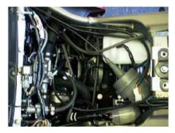
The **Actuator** (3) is located under the rear of the fuel tank. A **vacuum hose assembly** (4) is provided to connect the actuator to the engine. A vacuum fitting is provided to screw into the balance port to replace the original blanking screw.
