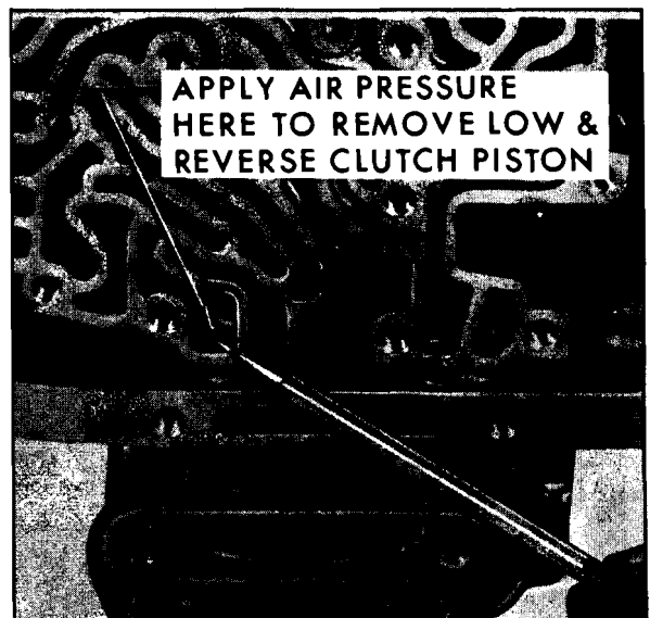
Fig. 7G-71 Using Air to Remove Piston
