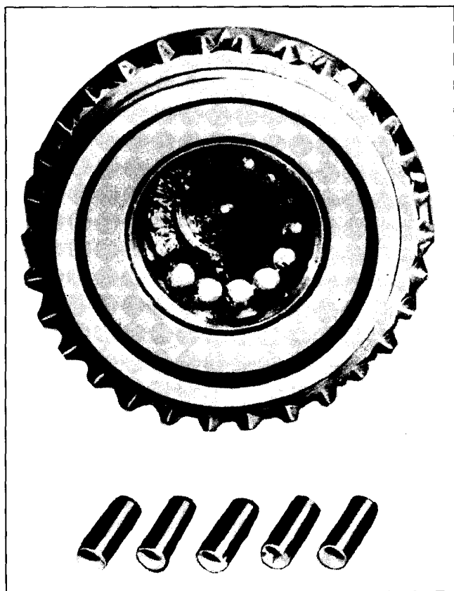
Fig. 7B-14 Loading Bearing Rollers into Main Drive Gear
