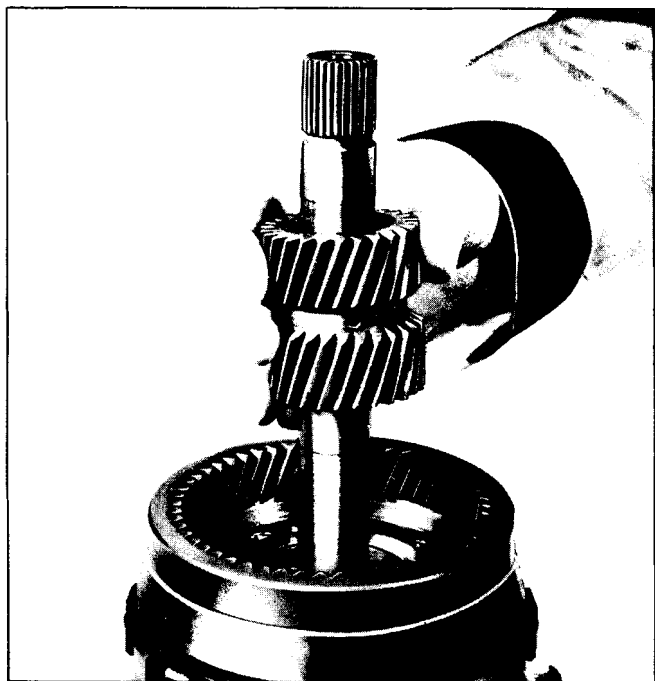
Fig. 7E-83 Removing Sun Gear
