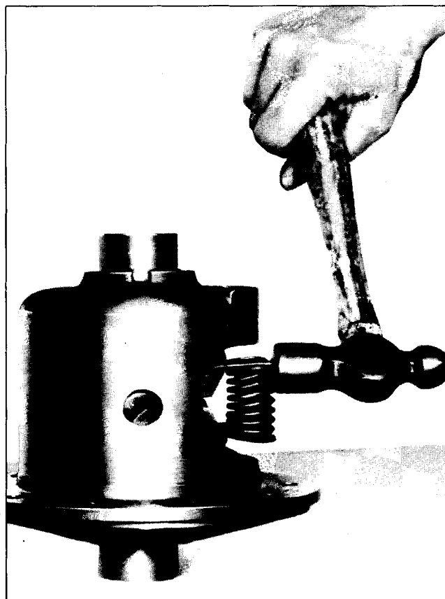
Fig. 4D-10 Installing Preload Springs and Retainers - Clutch Pack Type
