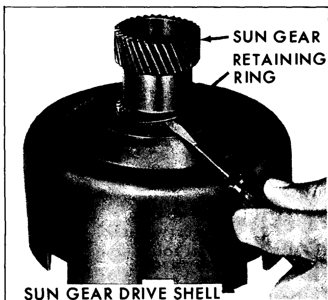
Fig. 7G-115 Removing Rear Retaining Ring
