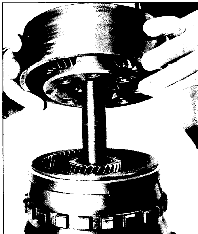
Fig. 7E-171 Installing Reaction Carrier
