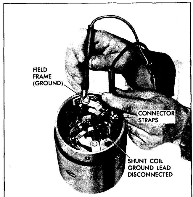
Fig. 6E-11 Testing Field Coils For Ground
