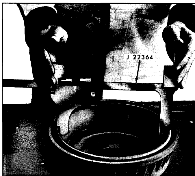
Fig. 5-14 Gauging Shoe to Drum Clearance
