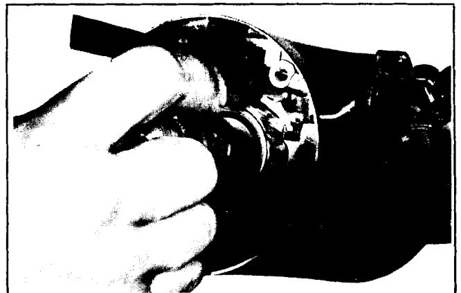
Fig. 9-27 Depressing Lock Cylinder Spring Latch
