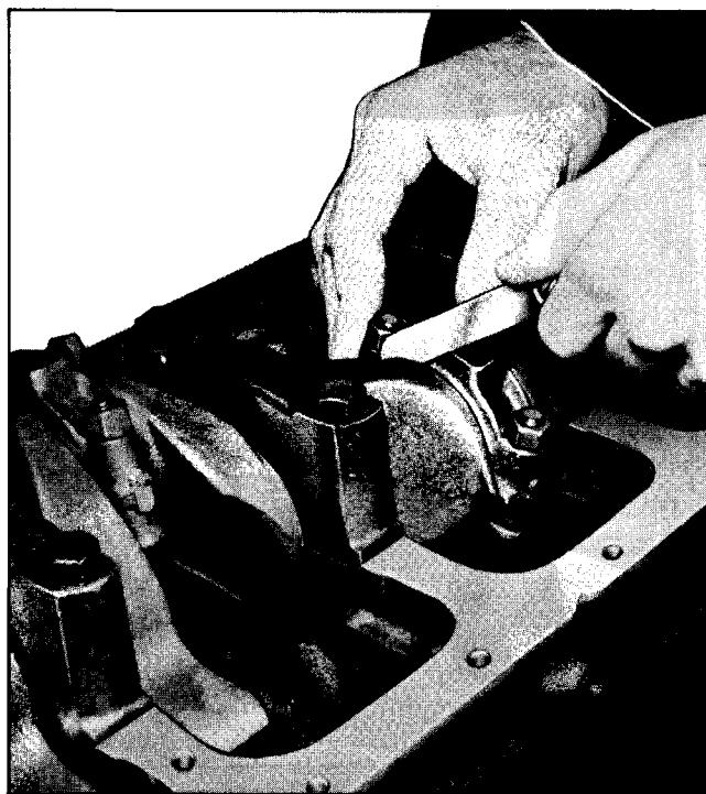
Fig. 6-58 Checking Connecting Rod Side Clearance
