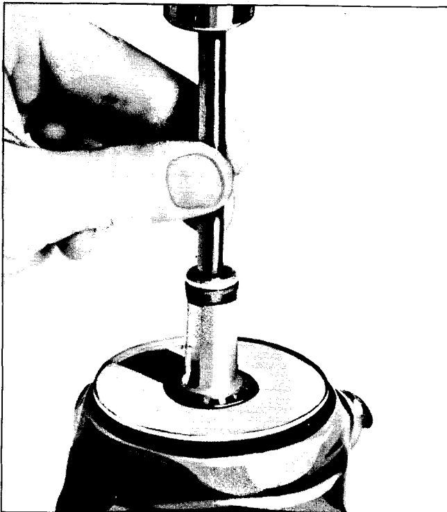
Fig. 4-43 Installing Expansion Plug Retainer
