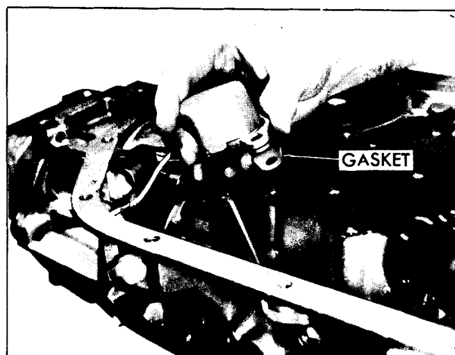
Fig. 7E-200 Installing Detent Solenoid and Gasket
