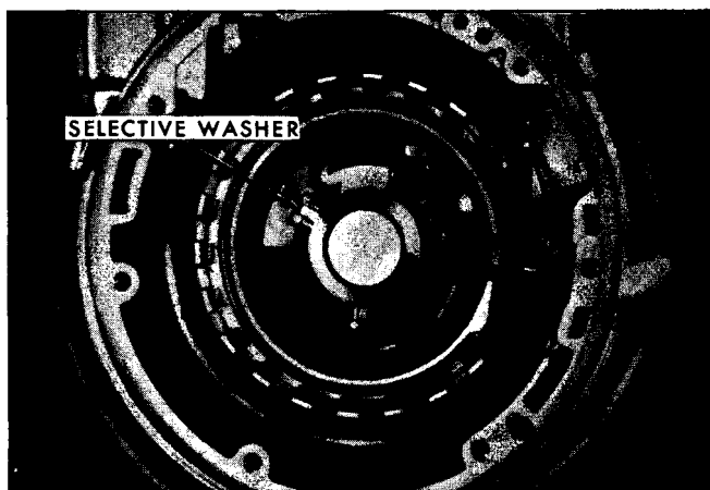
Fig. 7E-77 Location of Rear Unit Selective Washer
