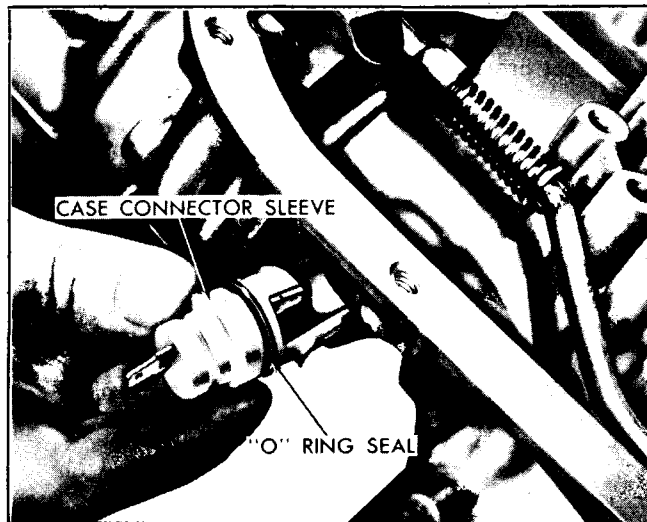
Fig. 7E-53 Removing Electrical Connector and O-Ring Seal
