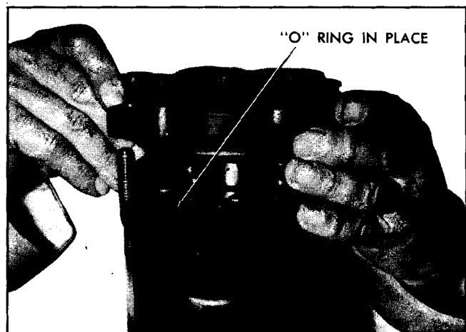
Fig. 1A-101 Installing Rear Head
