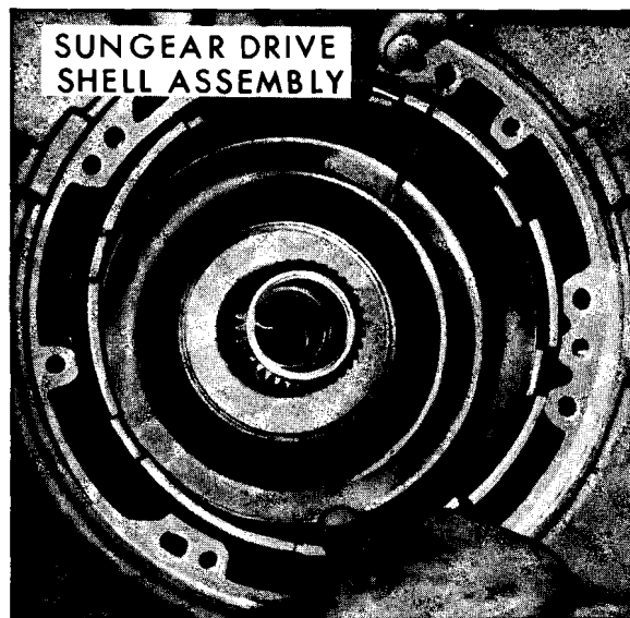
Fig. 7G-63 Removing Drive Shell
