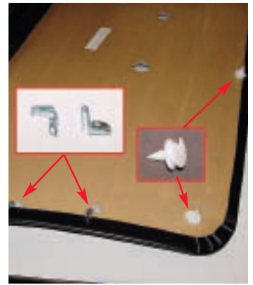
Photo #7: The power door lock switches were snapped into place with their supplied retainers. And now the door panel mounting clips, part #734046 , can be installed into the door panel, as well as the plastic button retainers, part #734045 . We found the clips install in the oval panel holes and the buttons screw into the round holes, by slipping the 90° corner under the cardboard and turning.
