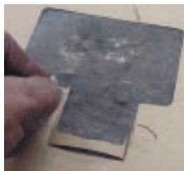
Photo #1: Project F2 has power windows. There was just enough left of our old door interior panel to determine the placement of the switch and we transferred this to the new watershield. The material was trimmed with a razor blade prior to installation.
