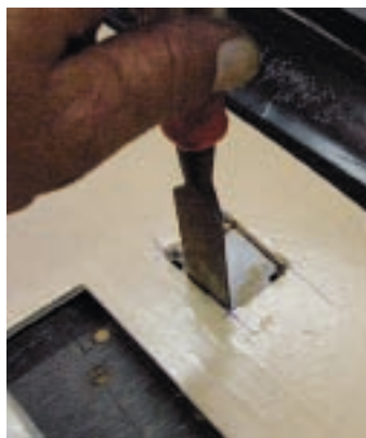
Photo #6: We used a disposable wood backer for the punch and pressed the door panel tightly to the backer before making our punch. We were concerned about slipping when making the final cuts with a knife so we elected to use a SHARP wood chisel and our cuts came out just fine.
