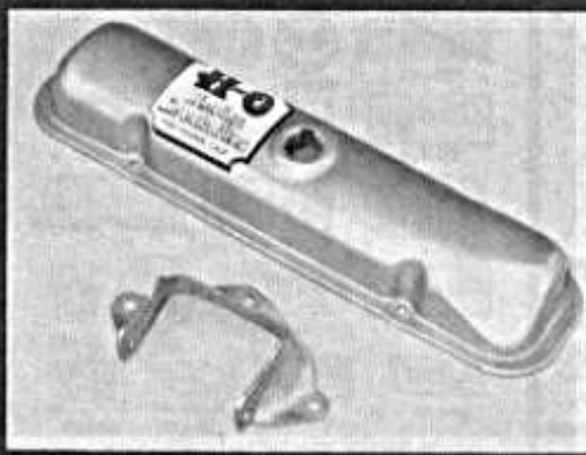
To provide clearance for the turbo exhaust, the right side of the engine is raised slightly with a special motor mount. Raising the engine creates an access problem with the left valve cover, so a modified valve cover is provided to clear the power brake.
